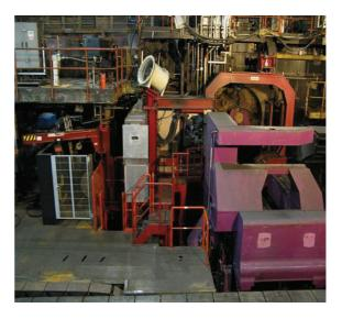
The M410 CH3A circumferential steel strapping machine can be equipped with a seal, seal less and also a spot weld version of the M410 steel strapping head for hot strip mill operations depending upon customer choice and application.
