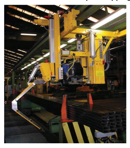
The M410-BRP-12 steel strapping machine is designed to secure square and hexagonal pipe or as here for profile bundles and can be easily integrated into customer stacking and packaging lines..
