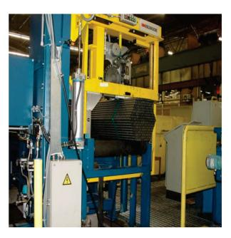
The BRP model shown here using optional AK200 head for Tenax PET polyester strapping of hexagonal tube bundles in a stationary machine version with the packages passing through the machine for strapping.
