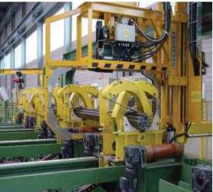
The standard M410-BRP-12 stationary machine and the M410-BRP-12-M indexing machine with fixed and opening strap chute systems located in customer specific pipe and bar section handling systems
